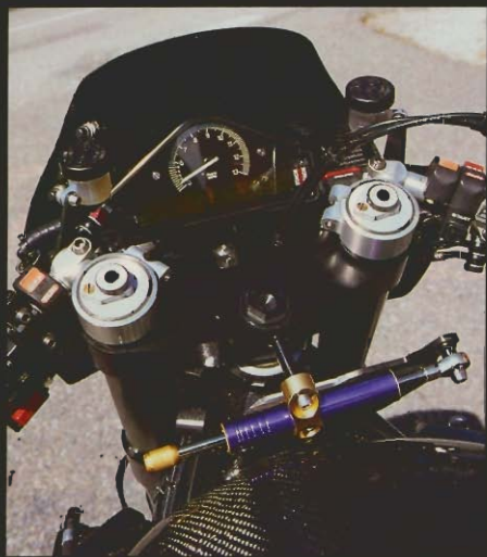
Speed-sensitive Hyperpro steering damper, digital Stack instrument console (with lap timer), carbon-fiber fly-screen and an empty, twisting road. Take our wives, please.
