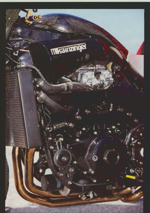
Big gulp: Giant carbon scoops ram atmosphere into a chamber inside the dummy carbon tank. Black, aluminum cross-plates help the frame handle the nearly 200-horse output, and a BMW car radiator keeps things cool.
